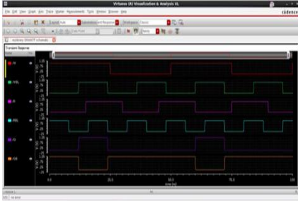
Fig5: Analysis of 7T SRAM
