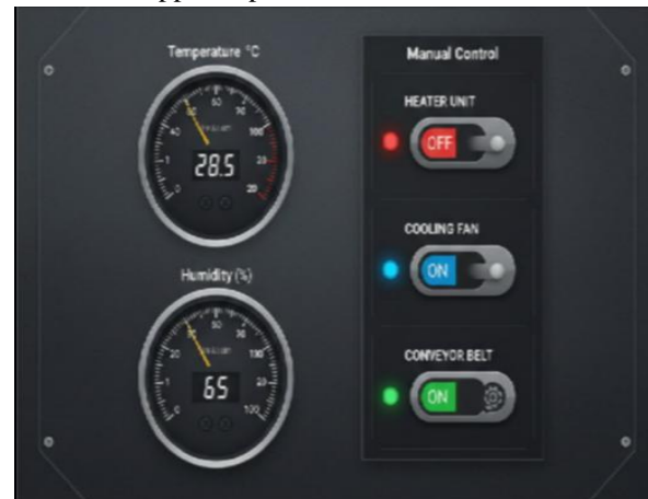
Fig. 4. Ignition SCADA Dashboard interface displaying real-time temperature gauges, humidity trends, and manual control switches for the loads.
