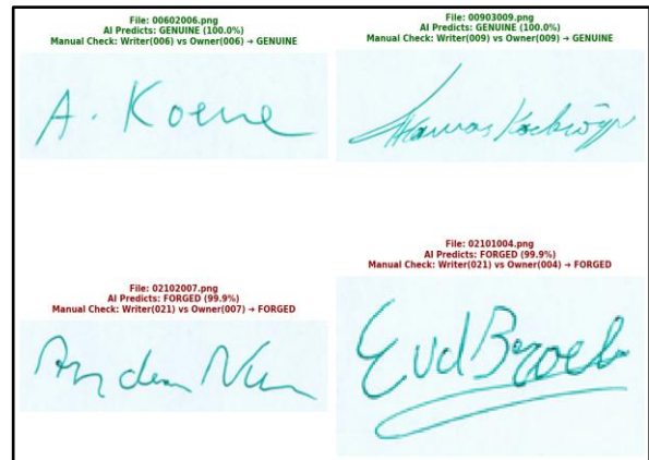
Figure 7. Backend Verification Grid Displaying AI Predictions and Manual Cross-Checking Validation.
