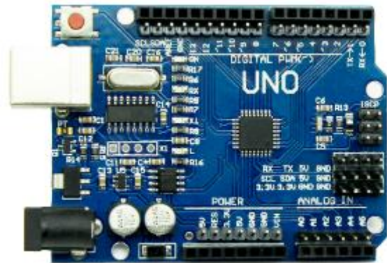
Figure: 4.1 Arduino uno atmega328p Microcontroller
