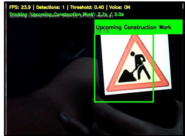
Fig. 11 Displaying the Message about Upcoming Construction Work Along with Confidential Value of 59.1%
