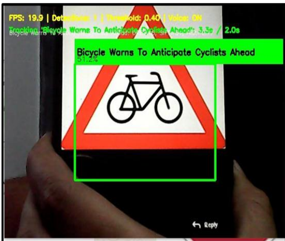
Fig. 9 Warns About there is Cyclist Ahead Along with Confidential Value of 51.2%
