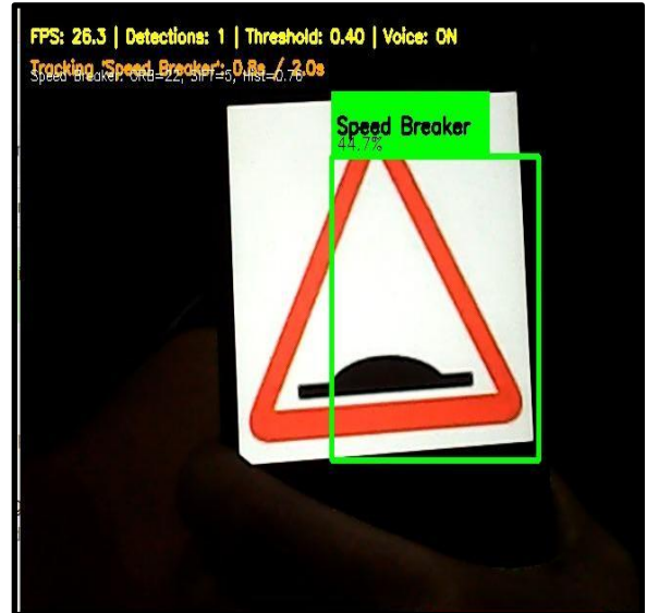
Fig. 5 Shows the Alert Message for Speed Breaker Detection Along with the Confidence Value Of 44.7%
