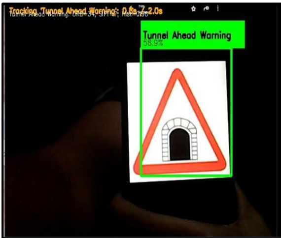
Fig. 14 Shows the Warning About there is Tunnel Ahead Along with Confidential Value of 58.9%
