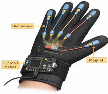
Fig. 4. Smart glove sensor placement showing Hall sensors mounted along the fingers and a magnet placed in the palm.
