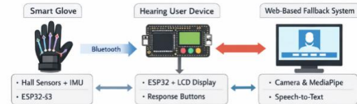
Fig. 1. Overall architecture of the proposed smart glove communication system.
