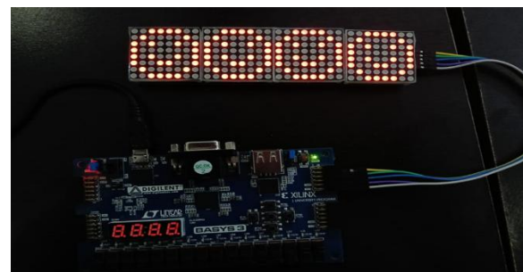
Figure 7: Hardware prototype: FPGA board interfaced with MAX7219 and 8x8 LED matrix.
