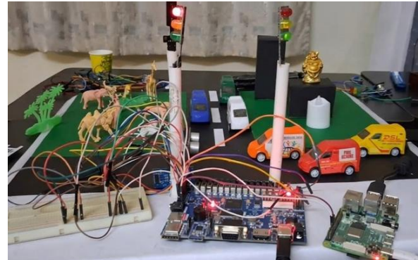
Figure 3: Hardware Implementation of Proposed Traffic Control System
