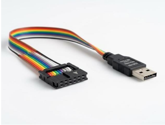
Figure 2: JTAG programming cable used for configuring the XC9572 CPLD
