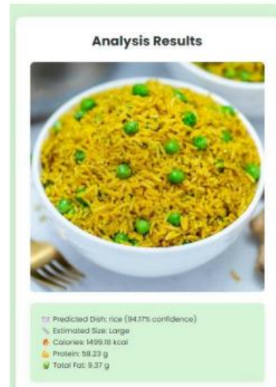
Fig. 4. Sample system output for a rice dish image with confidence score, nutrition breakdown, and diet recommendations.
