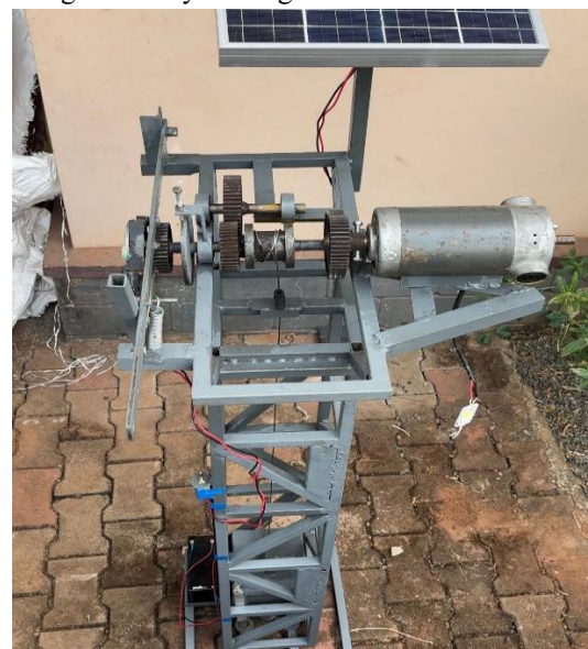
Fig 3. Fabricated model of the gravity battery
