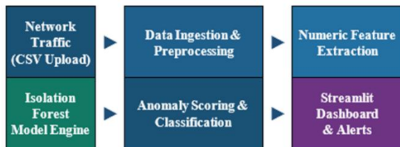
Fig. 1. End-to-end pipeline of the proposed AI-based cyber threat detection system.
