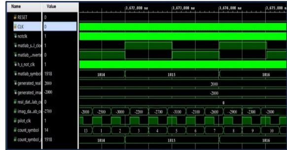
Fig.3 Waveform of MMSE channel estimation showing moderate variations with improved stability compared to LS
