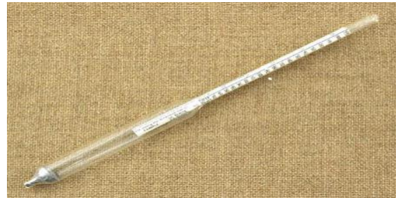
Figure 1 Hydrometer used for density measurement.
