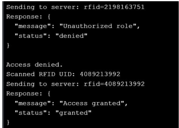
Fig: Serial Monitor output displaying staff access status based on RFID tag (Access Granted/Denied)
