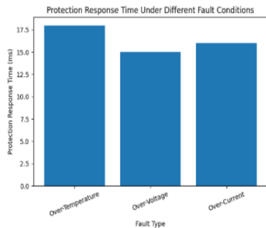
Fig. 3. Protection response time under different fault conditions.
