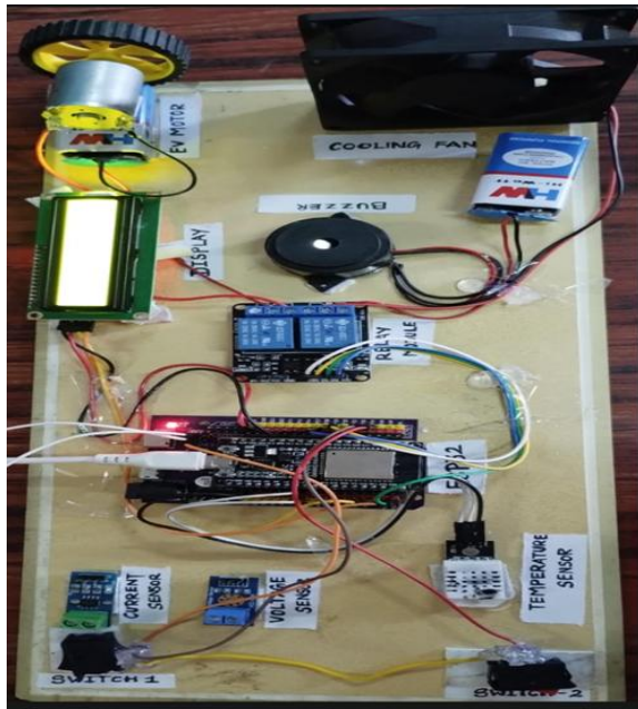
Fig. 2. Experimental hardware prototype of the proposed IoT-based EV charger monitoring and fire protection system.
