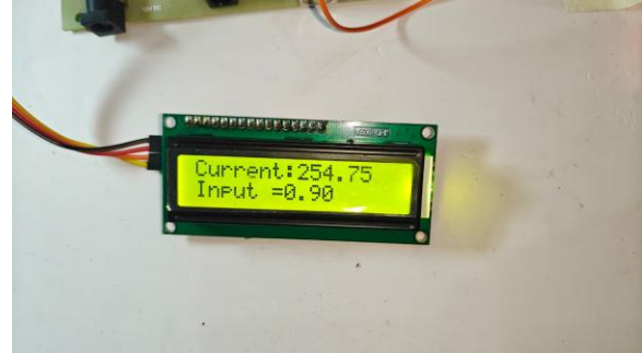
Fig. 6. Real-time current and input values displayed on the 16x2 LCD module.
