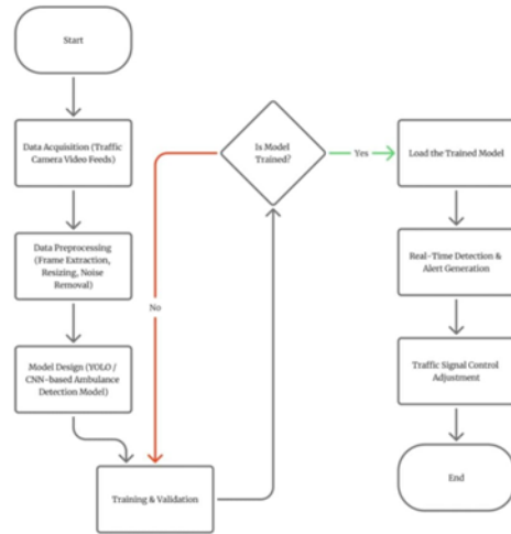
Fig. 1. Proposed smart traffic management system architecture of emergency vehicles.
