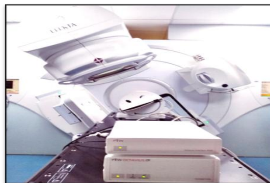
Fig:2 standard setup of patient specific QA with Octavius 4D
