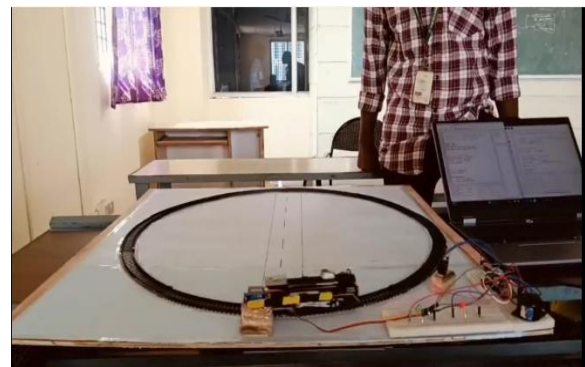
Fig. 8. Gate CLOSED – barrier horizontal, red LED lit, train approaching.
