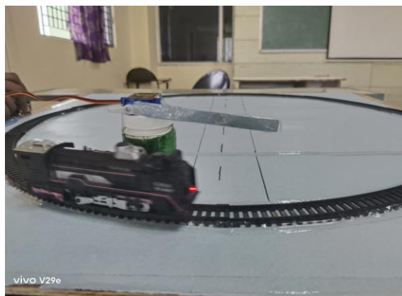
Fig. 6. Gate CLOSED - barrier horizontal, red LED lit, train approaching.
