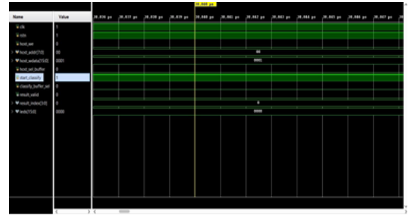
Fig. 14. Simulation waveform showing start classify output and input written data
