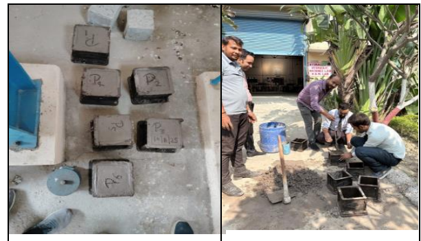
Fig. After Molding & during molding
