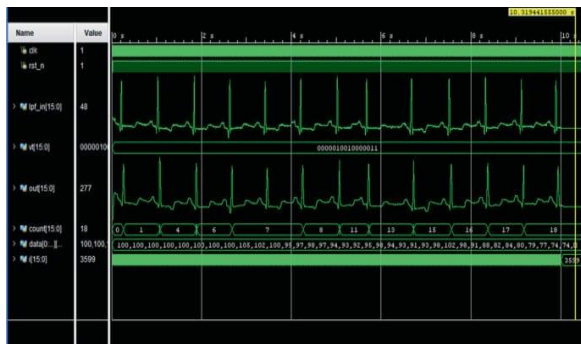
Fig 3. Simulated ECG output waveform obtained from FPGA implementation
