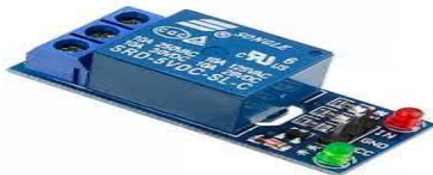
Fig. 6: Electromagnetic Switching Unit (Relay Bank)
