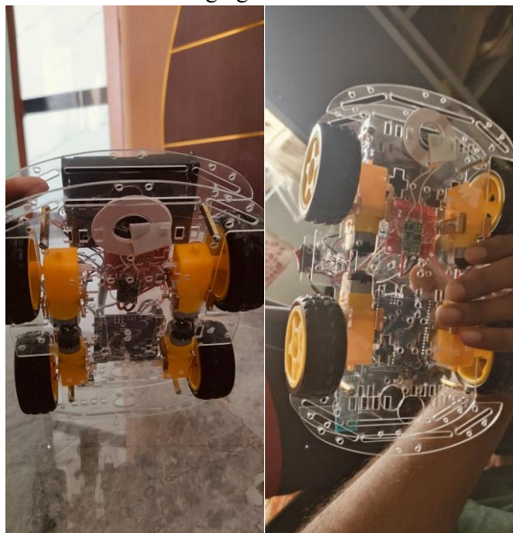
Fig.8. Robotic Car placed on Wireless Charging Pad for charging
