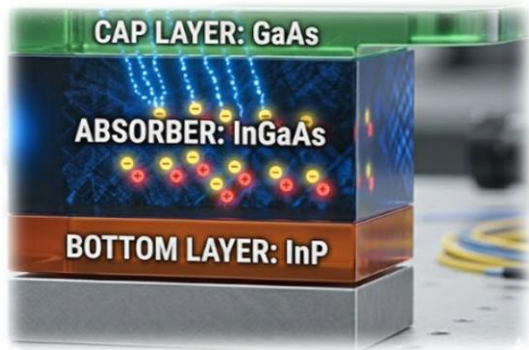
Figure 1: Proposed GaAs/InGaAs/InP Photodiode Structure
