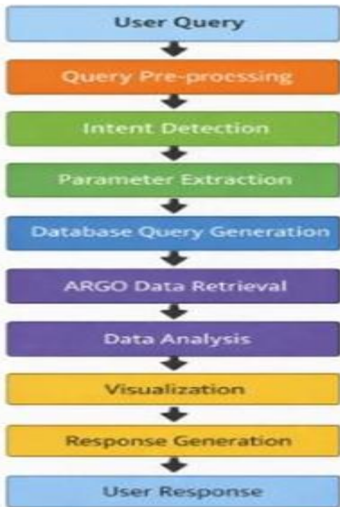
Fig. 3. Algorithmic workflow for conversational retrieval and analysis of ARGO oceanographic data in the FloatChat system.
