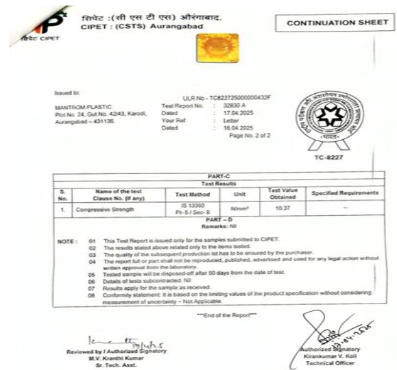
Fig. 1. Certified compressive strength test report of plastic-based grass block (CIPET).
