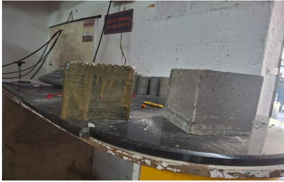
Fig 2 Concrete Cube with Carbon Fiber Wrapping
