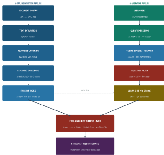
Fig. 1. Proposed Glass-Box RAG System Architecture – Dual-Pipeline Offline Framework
