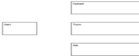
Figure 2: Fig. 4.2 — Use Case Diagram showing the User actor interacting with the three primary system use cases: Upload (dataset), Train (model), and Ask (question).
