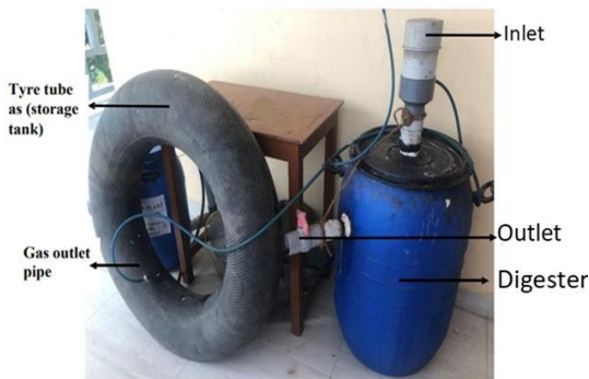
Figure 1: Pictorial representation of the biodigester set
