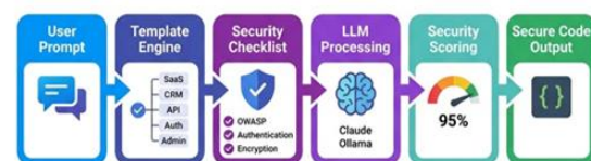
Fig. 3: M1 workflow: User Prompt → Template Engine (5 project types) → Security Checklist Injection (47 OWASP rules) → LLM Processing (Claude/Ollama/Simulation) → Post Generation SAST → Security Scoring → Annotated Code Output.
