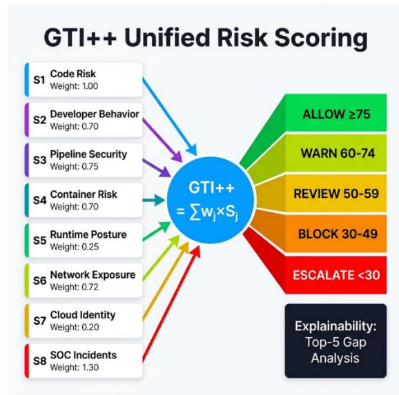
Fig. 12: GTI++ workflow: 8-dimensional scores weighted aggregation 5tier decision (ALLOW/WARN/REVIEW/BLOCK/ESCALATE) explainability with Top5 gap analysis.
