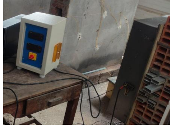
Fig: 20 Temperature Controller
