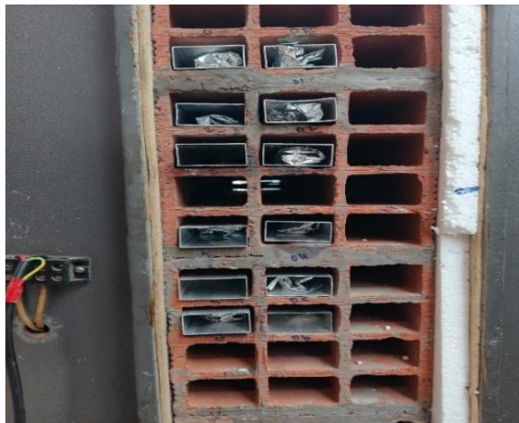
Fig: 11. Incorporating PCMs into bricks
