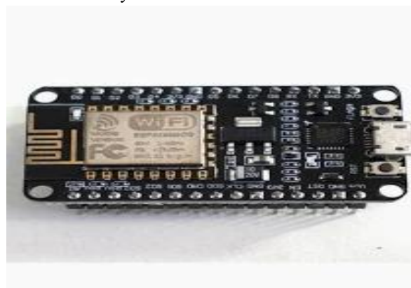
Fig 2: Shows the NodeMCU microcontroller board used for IoT applications and wireless communication.
