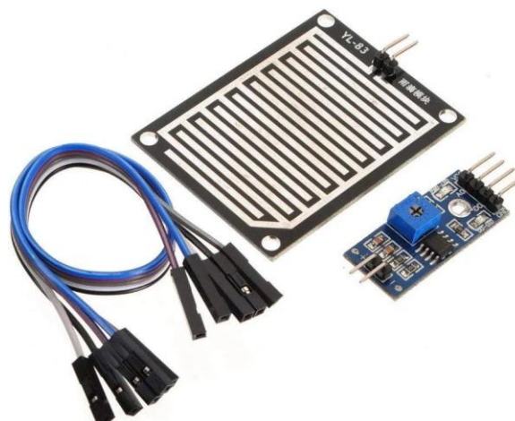
Fig 1: Shows the rain sensor module with detection plate, control board, and connecting wires.
