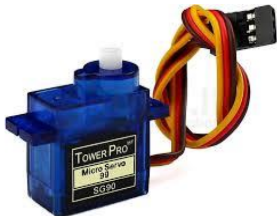
Fig 3: Depicts the TowerPro SG90 Micro Servo used for precise angular position control in embedded systems.
