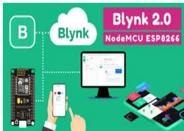
Fig 4: Shows the Blynk platform integrated with NodeMCU ESP8266 for wireless IoT-based control using a mobile application.
