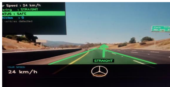
Fig. 1. System output on highway sequence. Both green lane boundary lines and transparent fill correctly detected. Steering: STRAIGHT. Speed: 24 km/h. STATUS: SAFE. Information box and bottom bar with steering wheel icon active
