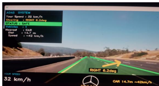
Fig. 3. CAR 14.7 m, ~42 km/h, adjacent lane — GREEN bounding box (SAFE, outside ego lane). RIGHT 6.2 deg steering. Your speed: 32 km/h. Pinhole model and dual-method estimator operating correctly.
