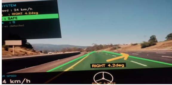
Fig. 2. RIGHT 4.2 deg: both lane lines and fill track road curvature without crossing. Slope-sign assignment crosses on this frame; position-based assignment does not
