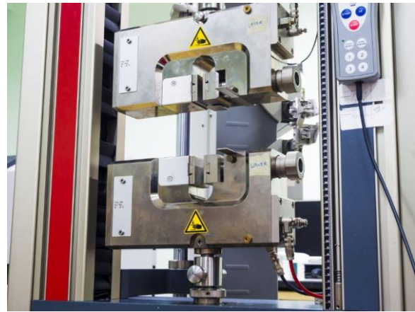
Fig. 4. Universal Testing Machine for tensile testing.
