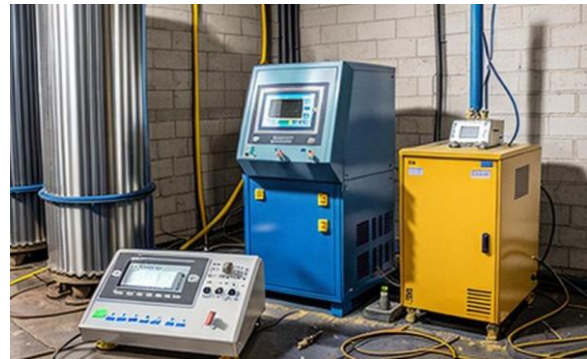
Fig. 5. Breakdown voltage test setup.
