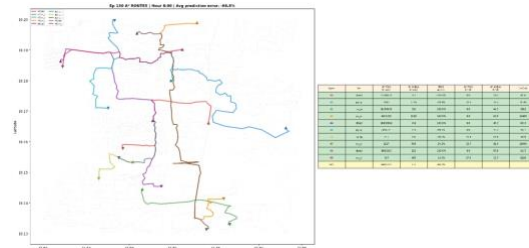
Fig. 2. Multiple routes forecasted using A* for multiple agents
