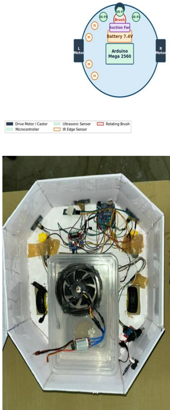
Fig. 2. Top-View Schematic of Robot Chassis and Component Layout.
