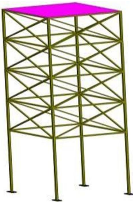
Figure 5: SOLIDWORKS model of the water tank stand.
