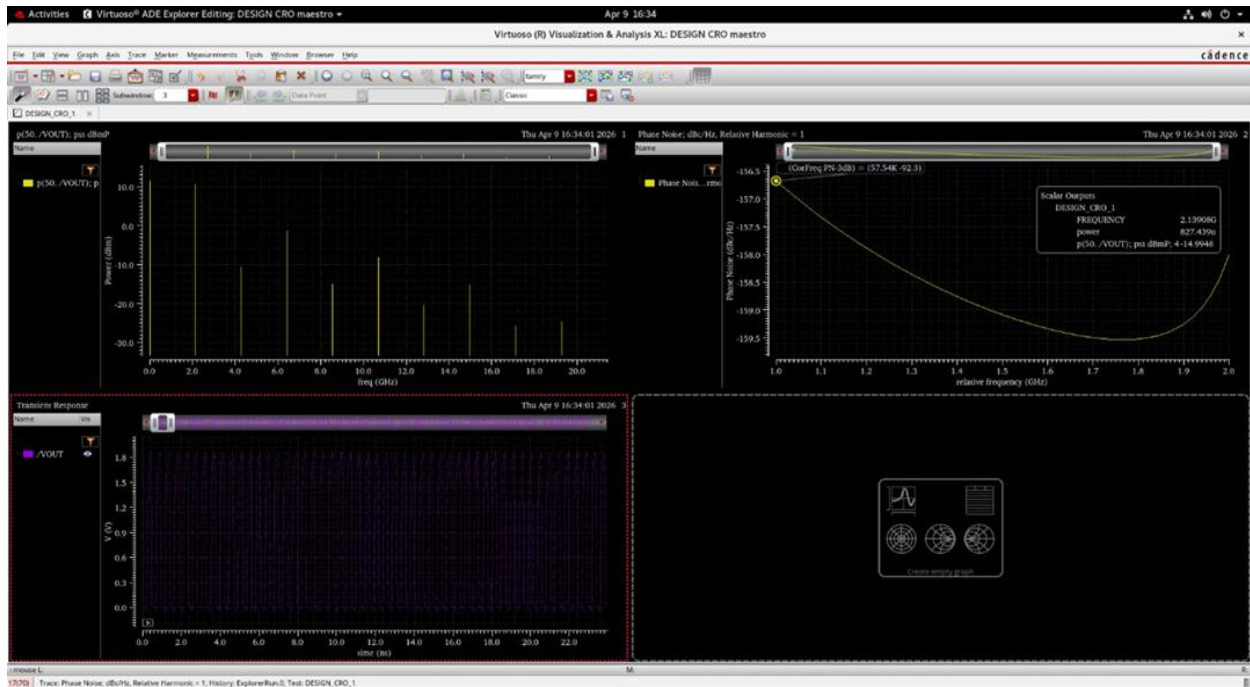
Fig. 8: Performance analysis of 7-stage CMOS ring oscillator
