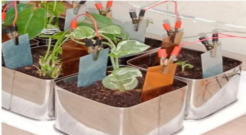
Figure 2: Pictorial representation of plant microbial fuel cell (P-MFC)
