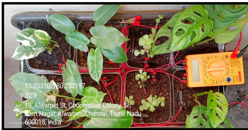
Figure 18: Pictorial representation of Series connection of P-MFC
