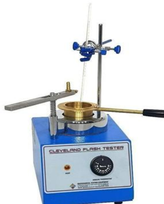
Fig 4: Flash and Fire Point Testing Machine This test determines the temperature at which bitumen gives off vapours (flash point) and catches fire continuously (fire point). It is useful for safety during heating.
