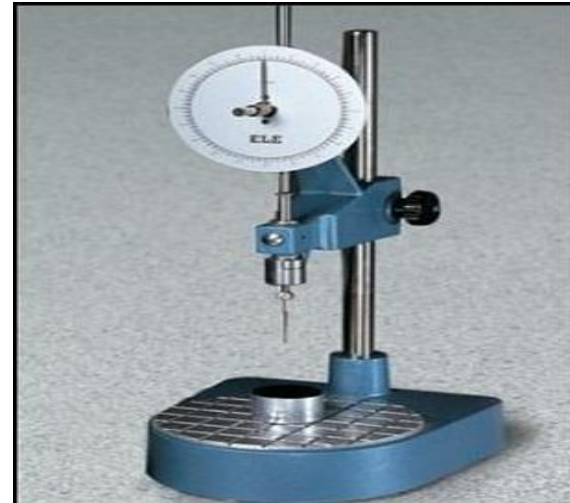
Fig 3: Penetration Test This test determines the hardness or softness of bitumen by measuring the depth of penetration of a standard needle under specified conditions.
