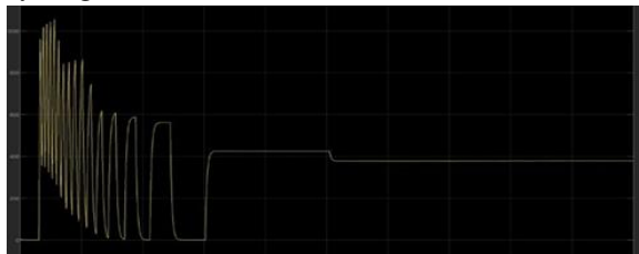
Fig. 9. Supercapacitor Power Output ( P_{SC} ) over Drive Cycle
