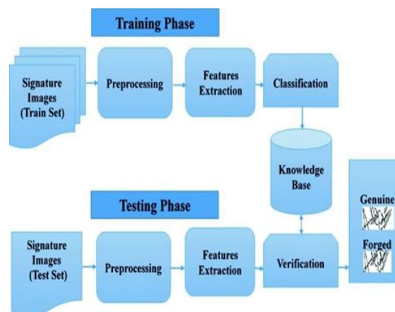
Fig.2. Architecture of Signature Fraud Identification
