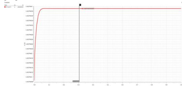
Fig. 4. Transient output response indicating settling near 1.43 V with a settling time of about 305 \mu\text{s} .
