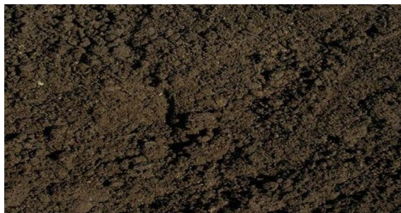
Fig. 3: Fine Texture of Air-Dried Black Cotton Soil After Disaggregation and Sieving (4.75 mm IS Sieve)
