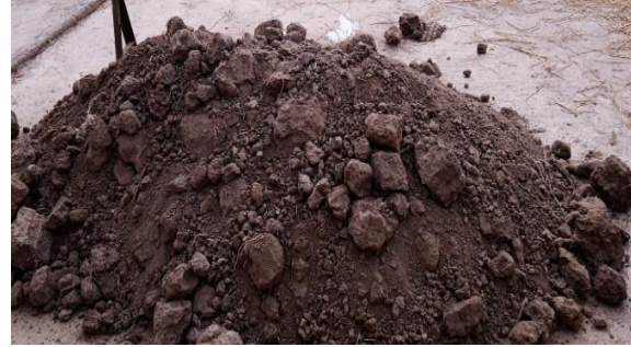
Fig. 1: Black Cotton Soil Sample Collected from Jalgaon, Maharashtra (Characteristic Dark Colour and Cloddy Texture)
