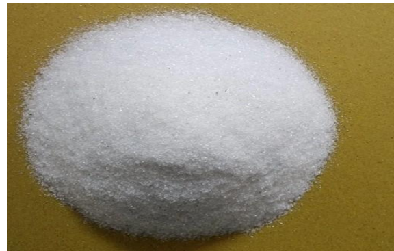
Fig. 2: Waste Glass Powder (WGP) Prepared from Discarded Glass, sieved through 75\ \mu\text{m} IS Sieve
