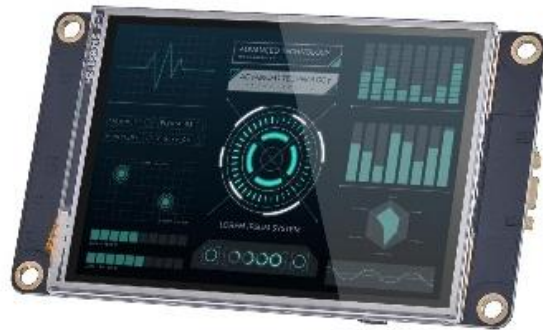
Fig.3. Enhanced Nextion display (NX3224K028)
