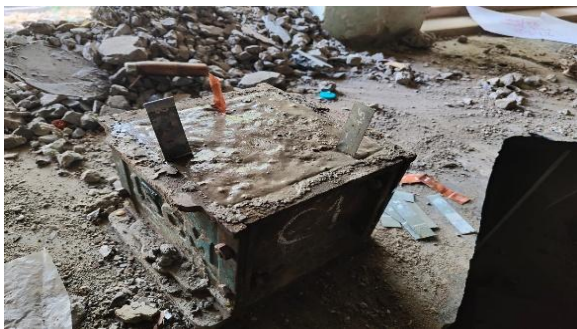
Fig. 3. Metal Strip Insertion in Concrete
