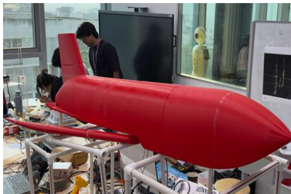
(b) Fabricated PLA article with segmented construction, alignment pins, mid-body wing panels, and cruciform fin surfaces fitted.
